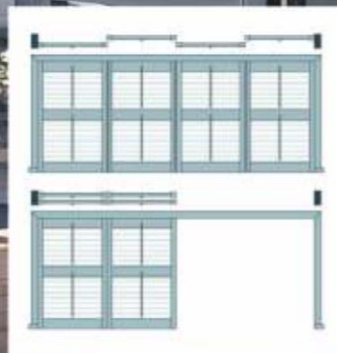
Rather than fitting shutters in the usual manner with frames and hinges, these shutters slide on a track.
